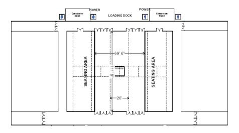
Rigging Info: 48' to the Low Steel (500lbs per panel point) 60' to the High Steel (500lbs per panel point)
